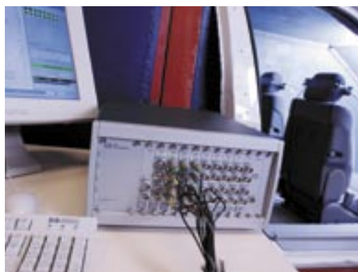
The LMS SCADAS 310 portable front end excels in performance and flexibility, with 10 slots for up to 40 channels or more in master slave configuration for high channel count testing.
