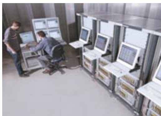
The LMS SCADAS 316 combines extremely high channel counts possibilities, real time processing capabilities and unmatched throughput performance.
